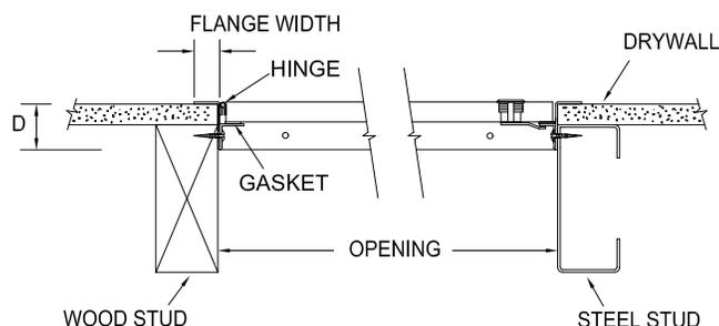
Model NGS met the performance criteria as per CSA A440-00 (windows) for an Air Infiltration of A-3 for both 75 Pa and 300 Pa, for Air Exfiltration the sample met an A-3 rating at 75 Pa and A-2 rating at 300 Pa. In Water Tightness by Static Pressure the door sample met a B-1 rating, subject to using an optional watertight mechanism, phone for details.
