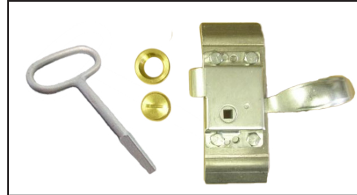
Zinc plated steel slam latch with removable tool on topside and a spoon handle on the underside; Standard with ASF, MT, and PFD floor doors.
