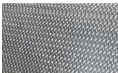
3/16" (4.78 mm) Steel Tread Plate
