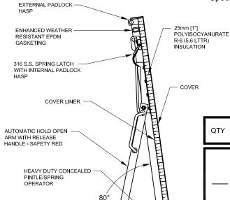
COVER MODEL MATERIAL COVER **CURB** LINER ALUM ALUM ALUM 12 ga 10 ga 12 ga RHA-15 ALUM 2.05mm 2.60mm 2.05mm
